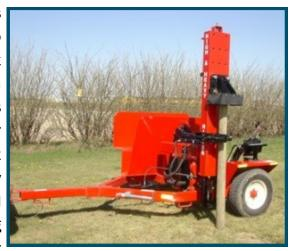
is the speed at which the posts can be installed. A normal 4-6" post can be driven in the ground in under a minute, even in dry or frozen ground. Another handy feature of the pounder is its ability to drive posts at an angle, this makes it capable of driving posts on steep terrain and installing angled vineyard end posts. Before you start your next fencing project contact the Prince Georges Soil Conservation District and we will get you started.
