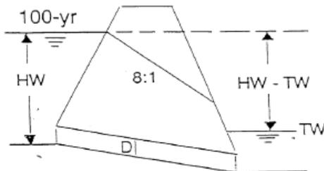
\* Use HW when TW is below the inlet invert elevation.
