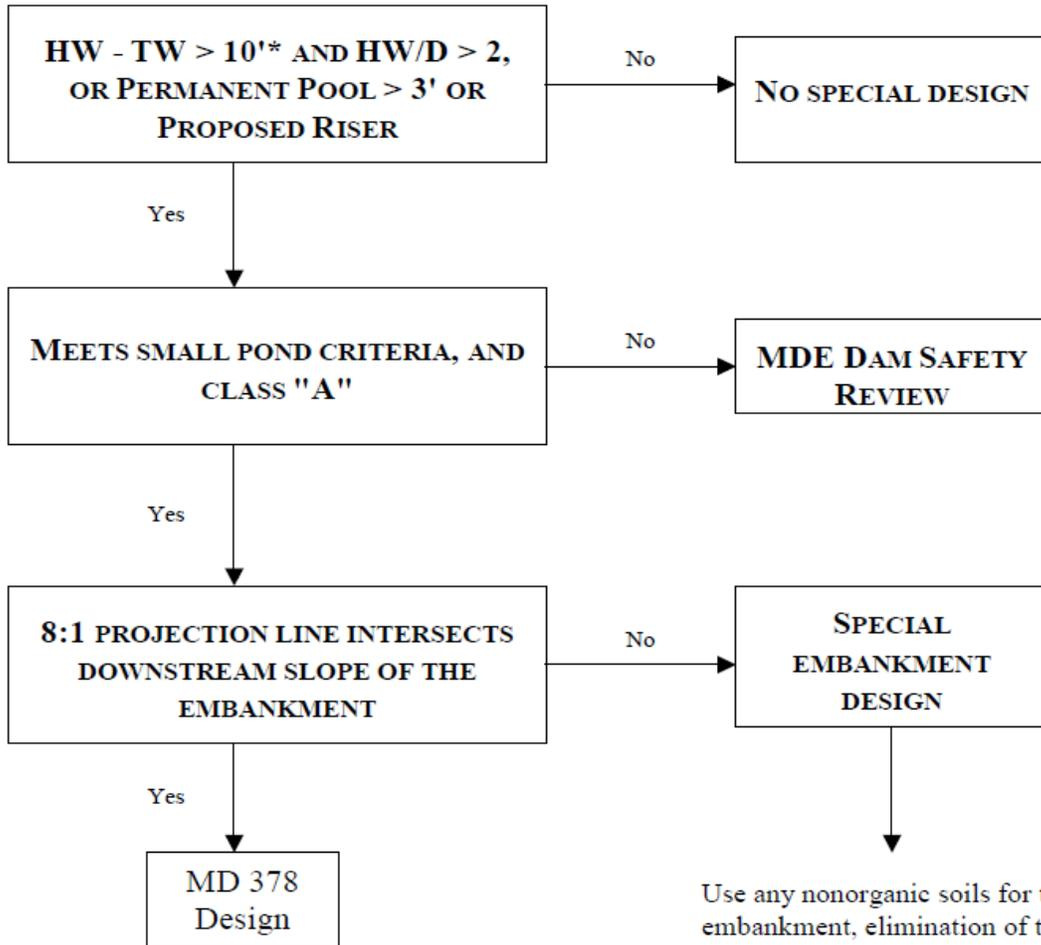
Use any nonorganic soils for the embankment, elimination of the cut-off trench and core based on approval of geotechnical engineer and acceptable to local jurisdictions.
